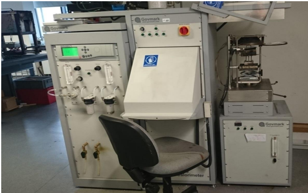
Photograph of Cone Calorimeter apparatus at the University of Central Lancashire, UK.
